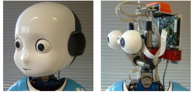
Fig. 3: ICub head (six degrees of freedom tilt, swing and pan for the neck) (Ruesch et al., 2008)
